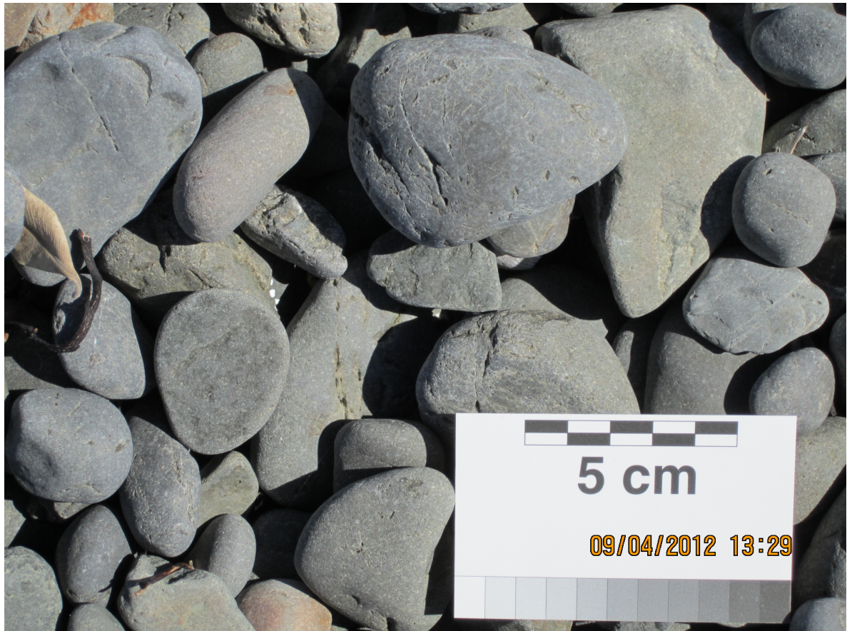
FIGURE 3: Photo of locally derived greywacke sandstone beach cobbles at Station OP-18 (Fig.2) on Waewaetorea Island which is representative of the greywacke gravels found on the beaches of the site.
